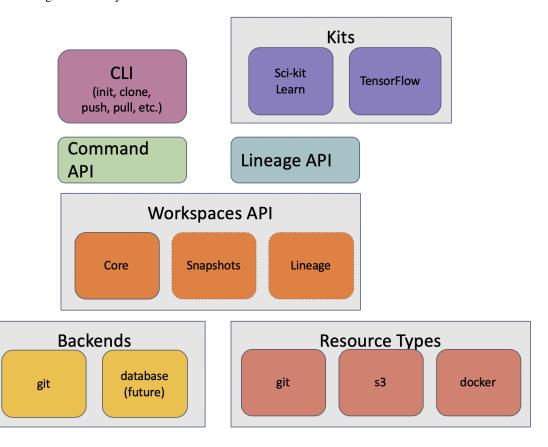
The core of the system is the Workspaces API, which is located in dataworkspaces/workspace.py. This API provides a base Workspace classes for the workspace and a base Resource class for resources. There are also several mixin classes which define extensions to the basic functionality. See *Core Workspace and Resource API* for details.
